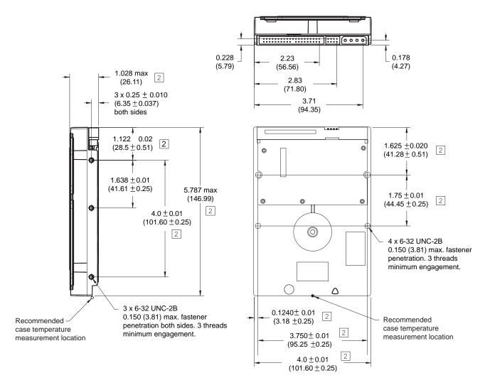
Figure 6 Mounting dimensions—top, side and end view
