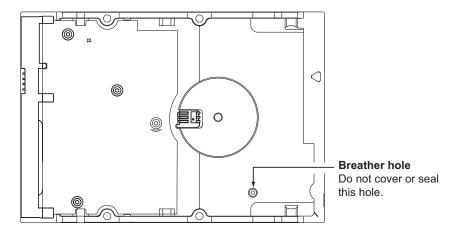
Figure 3 Breather filter hole location
