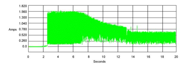
Figure 2 Typical 12V startup and operation current profile
